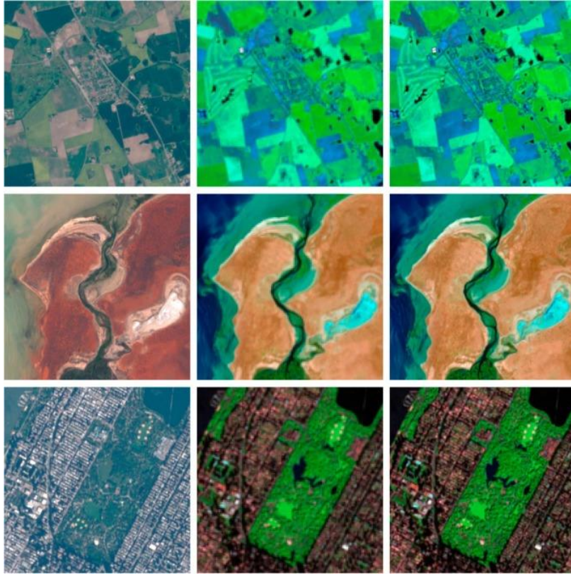
Figure 12: Visualisation of the Deep Sentinel-2 (DSen2) super-resolution model, performing 2\times up-sampling on real Sentinel-2 data. From left to right: true scene RGB in 10m ground sampling distance (GSD) (spectral bands B2, B3, B4), native 20m GSD spectral bands, and the super-resolved 20m GSD spectral bands (B12, B8a, and B5 as RGB) up-sampled to 10m GSD [18].
