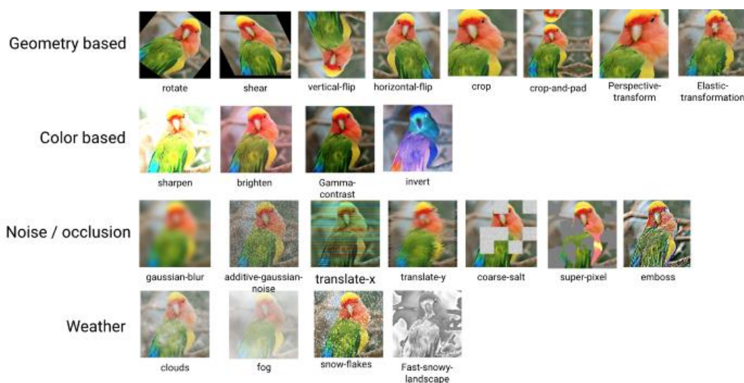
Figure 13: Depiction of a large collection of data augmentation (DA) techniques supported by ‘DeepAugment’; a DA solution, purposed to machine learning (ML) applications [119].
