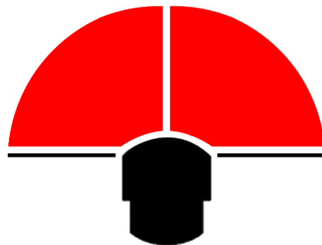
Figure 9: Pioneer P3-DX, front-most facing SONAR sensor partitioning visualization, used to apply the robot exiting, alignment behaviours. When exiting the inner-most room of the robots subjected environment.
