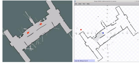
Figure 25: Particle filter ambiguity visualisation, particles formulate multiple densities reflecting uncertainty, concerning the structural symmetry of the robot's environment.
