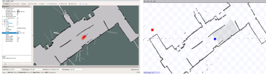
Figure 22: RVIZ tool visualisation, graphically depicting the estimated pose of the robot, published to the 'estimatedPose' data topic.
