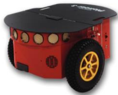
Figure 1: Depiction of the Pioneer P3-DX mobile robot [3].
