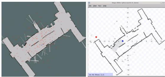
Figure 23: Particle filter initialisation visualisation, particles are uniformly distributed amongst the environment, initially.
