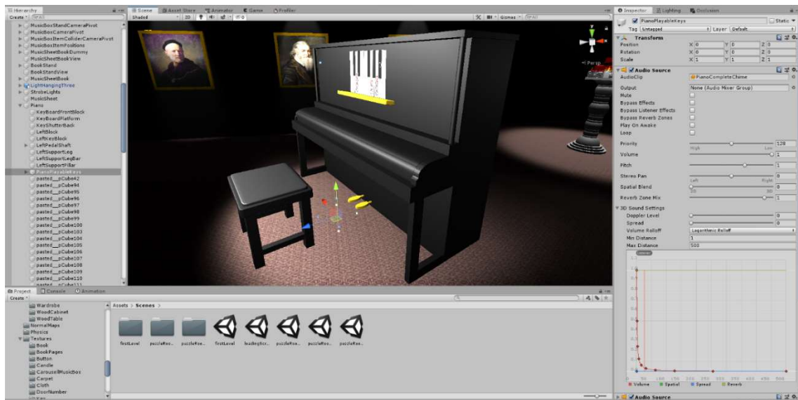
Figure 28: Puzzle room two, 'PianoPlayableKeys' object, numerous audio sources seen attached as components within Unity's inspector panel
